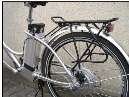
strong carrier rack brushless hub motor lock- and removable battery
