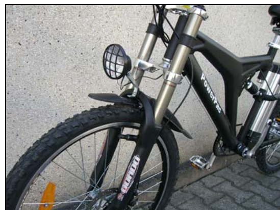
high quality suspension fork with adjustable compression stroke max. 115mm spring deflection
