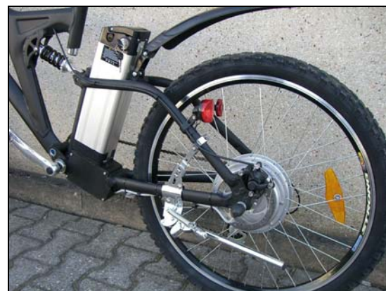
disk brakes and brushless hub motor
